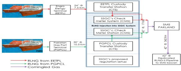
Figure 11: Process of RLNG transfer into the network system of SSGC
